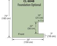
Furnace must be installed on a non-combustible surface or foundation that incorporates an enclosure that will prevent supply and return lines from any possible exposure to sunlight, fire, or physical damage that may be caused by an occurrence outside the furnace enclosure.
